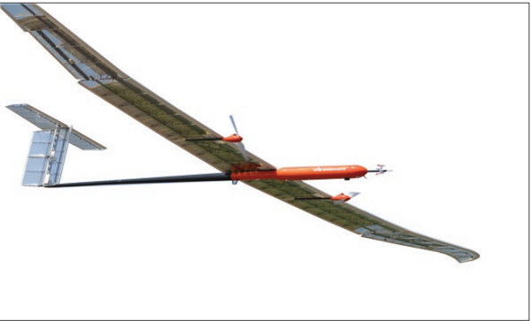
A high-altitude pseudo satellite equipped with the lithium-sulfur battery
